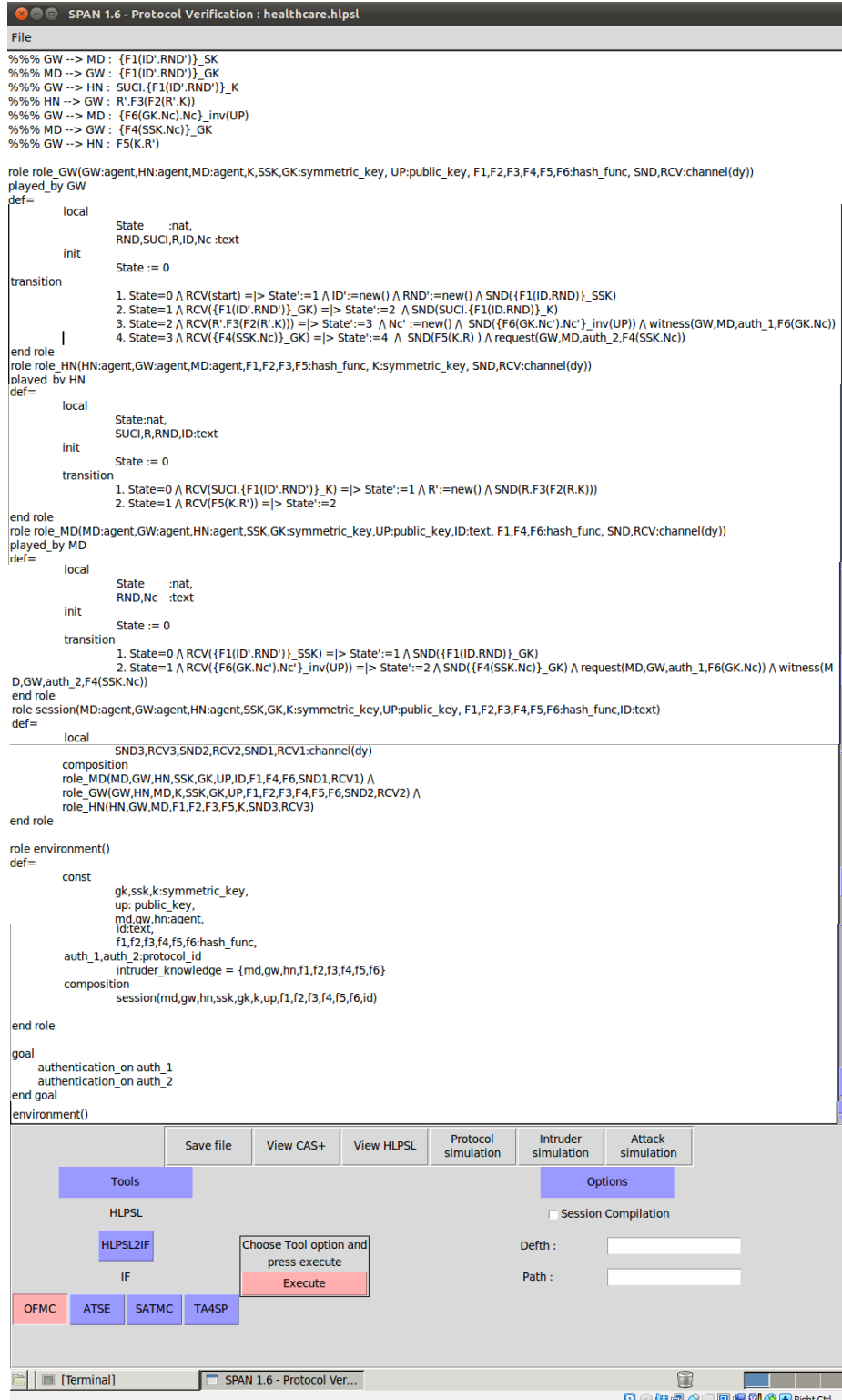
FIGURE 7: Program written for formal verification using AVISPA
